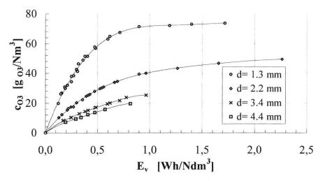
Fig. 4. Effect of specific energy density  $(E_v)$  on ozone concentration  $(C_{O3})$  at varied discharge gap (d), gas: air.
