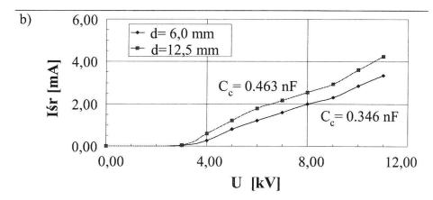
Fig. 2. Static operation characteristics of an ozonizer with a) PET and b) conducting packing.
