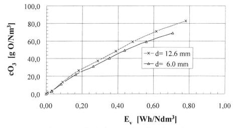
Fig. 5. Ozone concentration vs. energy density for an ozonizer with a wire packing, gas: air.
