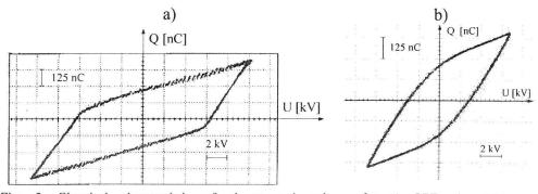
Fig. 3. Electrical characteristic of charge and voltage for a) PET, d= 2.2 mm and b) conducting packing, d= 6.0 mm, gas: air, f= 50 Hz.
