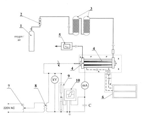
Fig. 1. Electrical circuit and a measurement system
